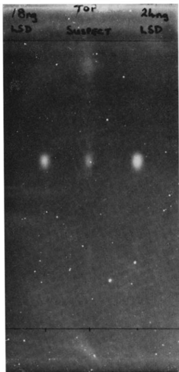
Fig. 5. TLC plate showing suspect LSD fraction viewed under UV light.
